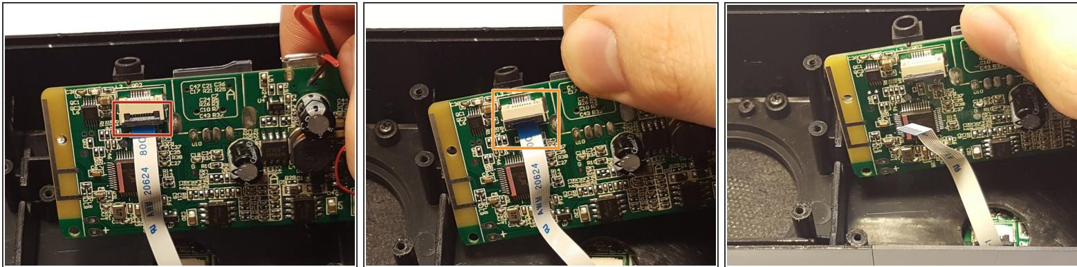
**i** You will finds a ribbon cable connecting the motherboard to the control interface circuit board.
